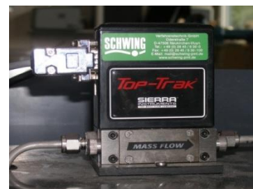
Casket with the SO 2 bottle and the electronic mass flow meter
