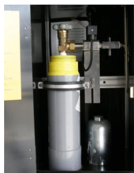
Casket with the SO 2 bottle and the electronic mass flow meter
