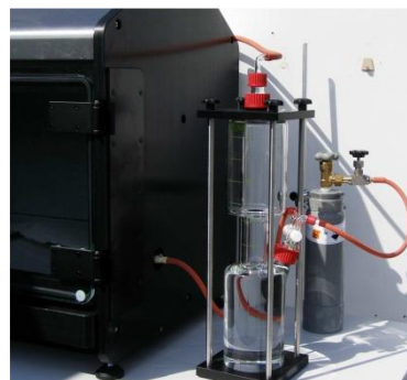
Front and side view of the glass cylinder for manual gas dosing
